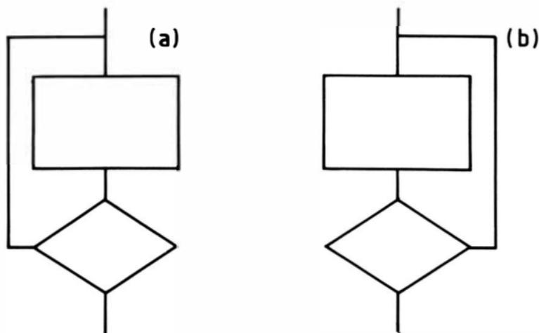
Fig. 2.5. Iteration: REPEAT UNTIL (a) true, (b) false.
