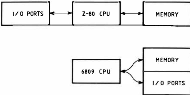
Fig. A.2. Z80 and 6809 memory and I/O ports addressing.
