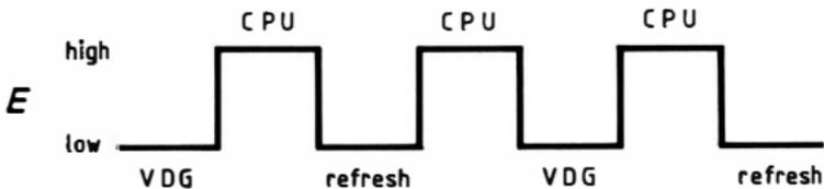
Fig. 4.1. CPU and VDG access to and refresh of dynamic RAM.
