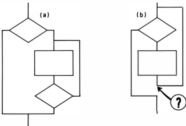
Fig. 2.6. DO WHILE true: (a) well structured, (b) pathological.
