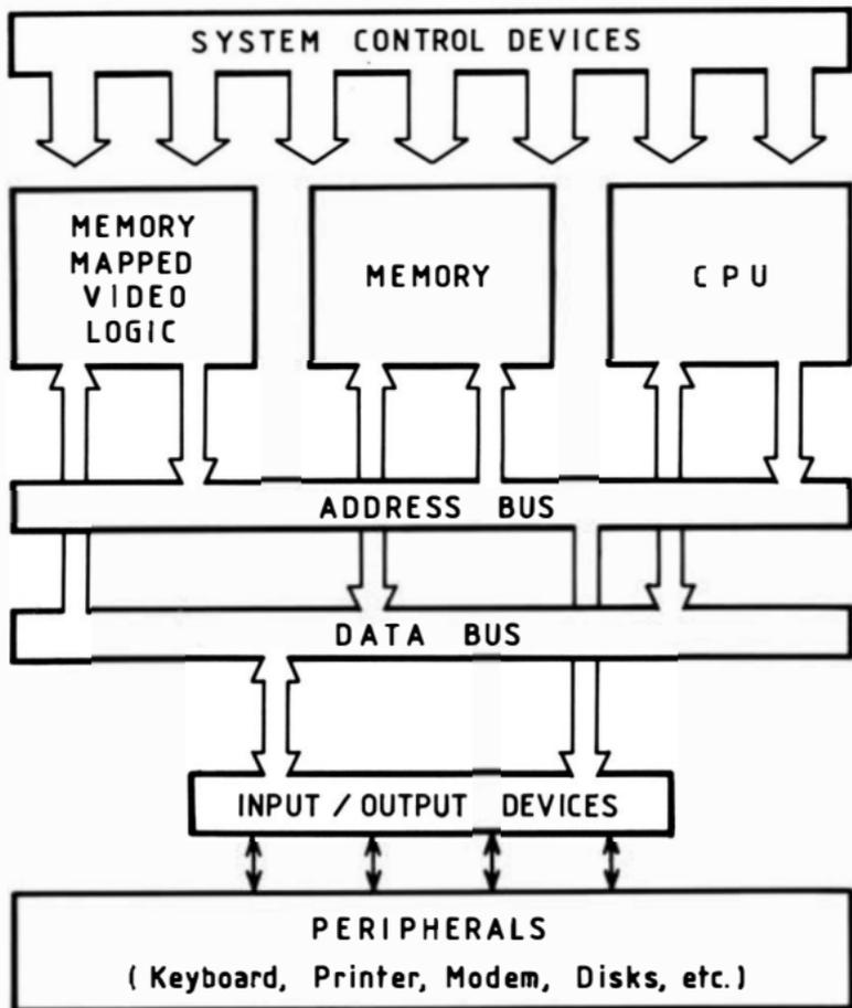
Fig. A.1. The main features of a computer system.
