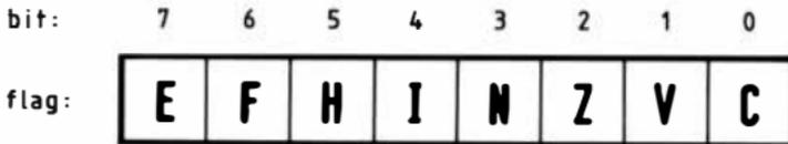
Fig. A.4. The 6809 condition codes register.
