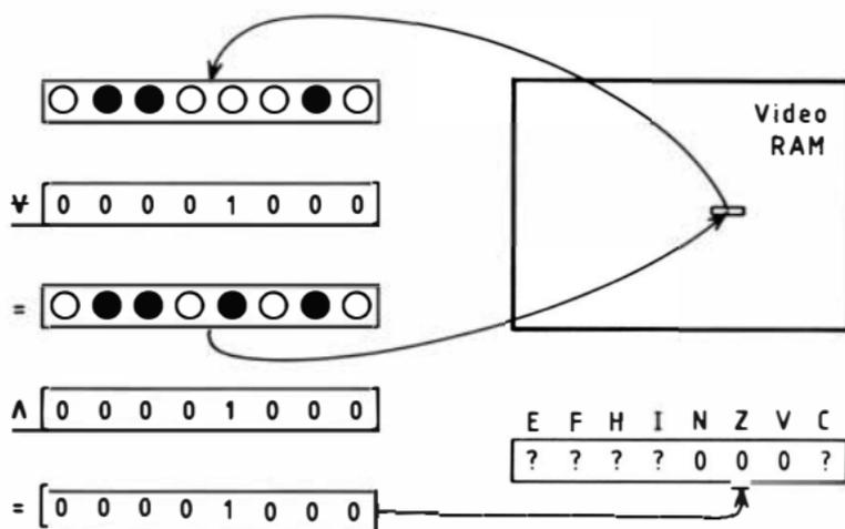
Fig. 6.1. Dot inversion and test in PLOT.
